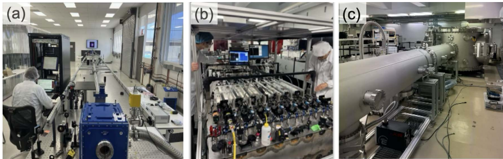
Fig. 6. (a) the 15m OEC at the Goleta facility in the US, (b) an 8-channel CBC utilizing fiber rod amplifiers under construction, and (c) the 15 m OEC developed and built at the BLF Japan Osaka site.
